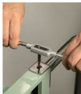
When hand tapping, always use tap wrench
